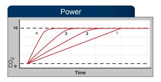
Power is a function of infusion rate of control gas. The higher the infusion rate, the faster to setpoint. Above: infusion rate #4>#3>#2>#1. Infusion rate is a function of control gas supply pressure. The higher the pressure, the higher the infusion rate. Maximum 25 PSIG provides 35 SCFH.
