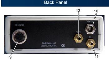
**9. Sensor Input Jack:** Locking sensor cable connects here. Finger tightened locking nut on cable plug secures it.
