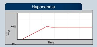
Hypocapnia is a relative term that means a lesser amount of CO<sub>2</sub> concentration (relevant to cell culture). In cell culture, 5% CO<sub>2</sub> is pretty standard practice. The ProCO<sub>2</sub> can create hypocapnia by infusing the CO<sub>2</sub> to a specific setpoint.
