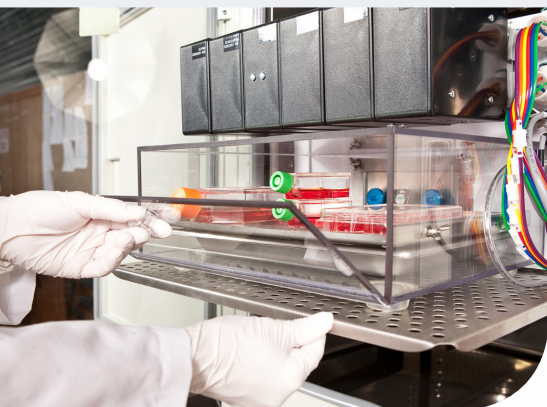
The GT series all use the same multipod adapter plate. This attaches to a C-Chamber and sits within your incubator.
