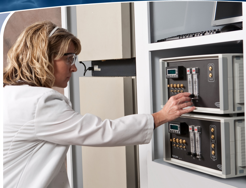
Single Chamber 0-400 PPM CO Control
