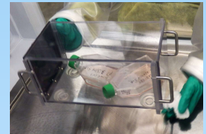
Figure 1d. The Transferable Conditioned Culture Chamber Atmosphere is Conditioned by Isolator During Cell Handling. After cell culture vessels were transferred from each TCC into the processing chamber, the TCC door was left open to condition the atmosphere inside. The cultures were replaced in the TCC after cell handling and the chamber was magnetically sealed for transport out of the isolator and back to the external incubator.
