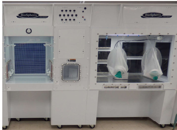
Figure 1. Experimental Design. Routine cell processes (cell thawing, media change, and cell harvest) were mimicked using TSB media (BioMerieux, St. Louis, MO). All operations were performed inside the Xvivo System including centrifugation (not pictured), incubation of the mock cultures between processes, and harvest of the surrogate cell product into sterile vials. Surfaces in the Xvivo System were sampled using contact plates after each process. Three full trials were performed. Materials were surface disinfected with SporKlenz (Steris, Mentor, OH) in the Laminar Flow Hood (left) and moved into the Process Chamber (right). All gases were medical-grade, tanked, and continuously HEPA-filtered.
