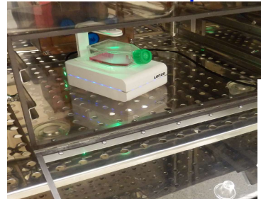
Figure 1. Experimental Set-Up. Lonza human bone marrow MSC cells were thawed under physiologic conditions (37°C, 5%CO 2 , 5%O 2 ) and immediately split into two conditions: Lonza hMSC Basal Medium plus MSCGM, hMSC Singlequot Kit, and Lonza Trypsin/EDTA for MSC, and Lonza DPBS w/o Ca/Mg (Lonza, Cologne, GmbH). One flask of each set was used for monitoring with the Lonza CytoSMART microscope and three were used for cell counts. Cells were monitored for cell density and the subcultured when no more than 80% confluent. Medium was exchanged every 3-4 days. Cells were trypsinized, washed, and counted at each passage. Cell coverage data and time-lapse photomicrographs were provided by the CytoSMART. Statistical overlap between group cell counts were assessed using Excel (Microsoft, USA).
