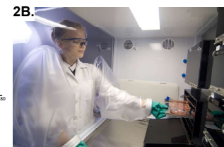
Figure 2. Cell Processing Atmosphere is Effectively Separated From Room Air. Full-time particle detectors in the barrier isolator did not detect particles leaking from room air into cell processing chamber (2A). Small numbers of non-viable particles were generated by motion of the integrated sleeves and gloves during normal cell handling (log-scale inset) (2B). Environmental monitoring using touchplates and an air sampler that drew air over a touchplate during cell handling detected no viable CFUs in the cell processing chamber (Table 2) over three sessions.
