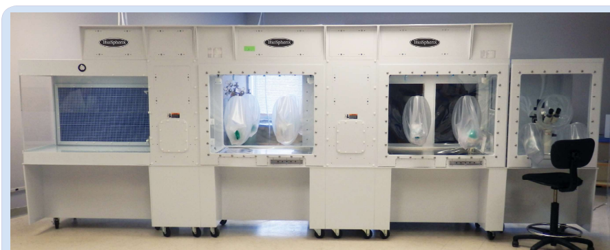
Figure 1. Experimental Design. All processes were performed in the Xvivo System which provides a completely controlled atmosphere from filtered, tanked gases. No room air is inside. The atmosphere is continuously HEPA filtered for particle control to ISO 5 levels during cell processing. The temperature of the floor and air of each chamber can be controlled to constant 37°C. The black doors cover integrated cell incubation chambers. Materials were brought into the system through the laminar flow hood on the left. Buffer chamber air locks exchange any entering room air with tanked gases before materials were imported. Before processing, probable risk surfaces inside the Xvivo and all imported materials were surface disinfected with SporKlenz RTU (Steris). Sterile vials were filled with color-changing highly permissive TSB broth (BioMerieux). After pre-process cleaning, touchplates were used to assess probable risk surfaces for microbial contamination. This was repeated before post-process cleaning. During vial filling, an air sampler was used to draw processing chamber air across a touchplate. All vials and touchplates were incubated for 14 days or 48 hrs respectively and vials were assessed at Days 7 and 14 for contamination analysis. n=3 trials of 96-100 vials each. Positive controls were exposed to the room environment outside the Xvivo System. Negative controls were not exposed at all.
