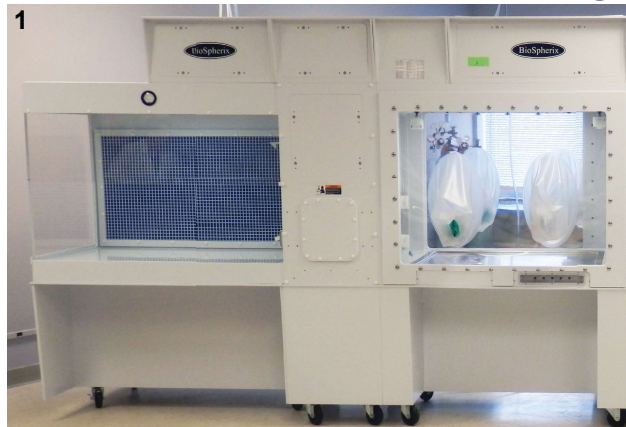
Figure 1. Experimental Set-Up Mock fill/finish processing was performed in an Xvivo System barrier isolator with color-changing tryptic soy broth (Biomérieux) that is highly permissive for microbial growth. Air inside the system was from tanked, medical-grade gases and was subjected to constant HEPA filtration with a continuously-recirculating air cleaner (CRAC) system. All entering materials were manually wiped with gauze dampened with SporKlenz (Steris, USA) for surface disinfection in a laminar flow hood (LFH), the chamber on the left, with HEPA-filtered room air. Materials passed through an airlock (buffer chamber, not visible) which changed entering HEPA-filtered room air to tanked gases. All open processing was performed in the double-sided processing chamber on the right side. With prepared TSB, bagged sterile vials with caps and seals were imported. After vial filling, the vials were exported from the barrier isolator and incubated in a room air incubator for 14 days. During vial filling, an air sampler pulled processing chamber air across a contact plate. After each trial, Rodac environmental monitoring contact plates were applied to the floor in integrated places, and each fingertip of each set of integrated system gloves. Six separate processes were performed with 100 vials each for a total of 600 vials tested including 1 positive control injected with 0.1ml of non-sterile water for each batch.
