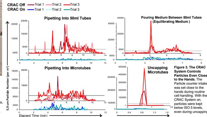
**Figure 3. The CRAC System Controls Particles Even Close to the Hands.** The Particle counter intake was set close to the hands during routine cell handling. With the CRAC System on, particles were kept below ISO 5 levels, even during uncapping.
